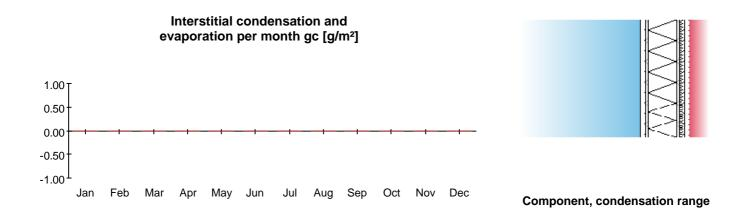
Condensation Risk Analysis calculations according to BS EN ISO 13788 are used as a guide in predicting interstitial condensation. This methodology uses some simplifications of the dynamic processes involved and subsequently does have some limitations. For further information the user is advised to follow the prescriptive guidance in BS 5250:2021 Management of moisture in buildings – Code of practice & BRE Information Paper:IP2/O5 (Feb. 2005) 'Modelling and controlling interstitial condensation
